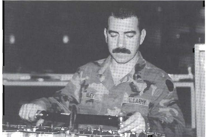
Sgt. Gene Riley, Co. B, 103rd Forward Support Battalion, rebuilds a humvee engine at the Combined Support Maintenance Shop.
