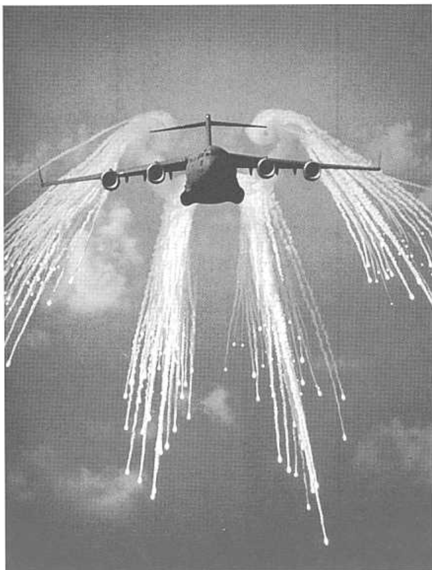
Photo is courtesy of McDonnell Douglas An Air Force C-17 Globemaster dispenses flares during testing of its infrared-seeker defense system at Eglin AFB, Fla. The first operational C-17s from Charleston AFB, S.C., arrived at an Arabian Gulf region air base Oct. 15 and marked the first deployed mission for the Air Mobility Command's newest airlifter.
