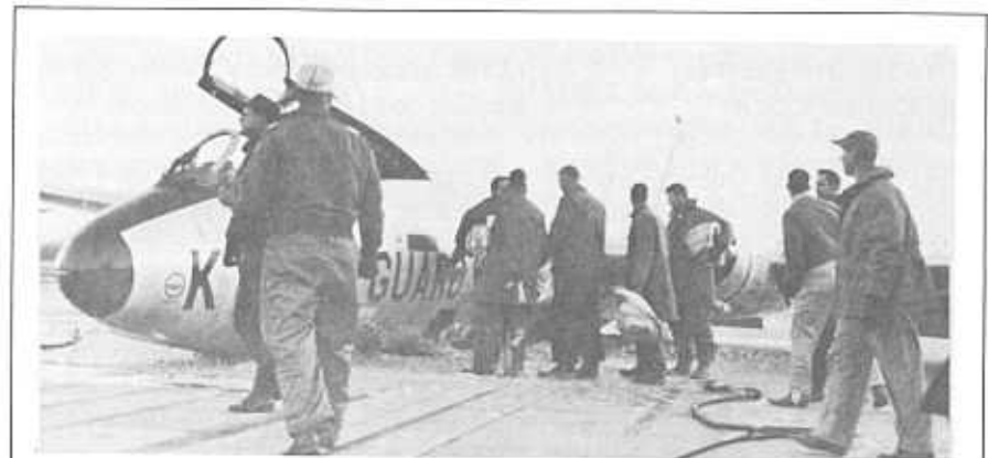
Photo is from the KyANG historical archive BELLYLANDING -- Lt. Col. James Pickett found his wheels wouldn't go down as he attempted to land at Standiford Field in 1962. Quick thinking and good work by ground crews provided the way. Foam was laid and Pickett was able to belly in his RB-57 Canberra aircraft.
