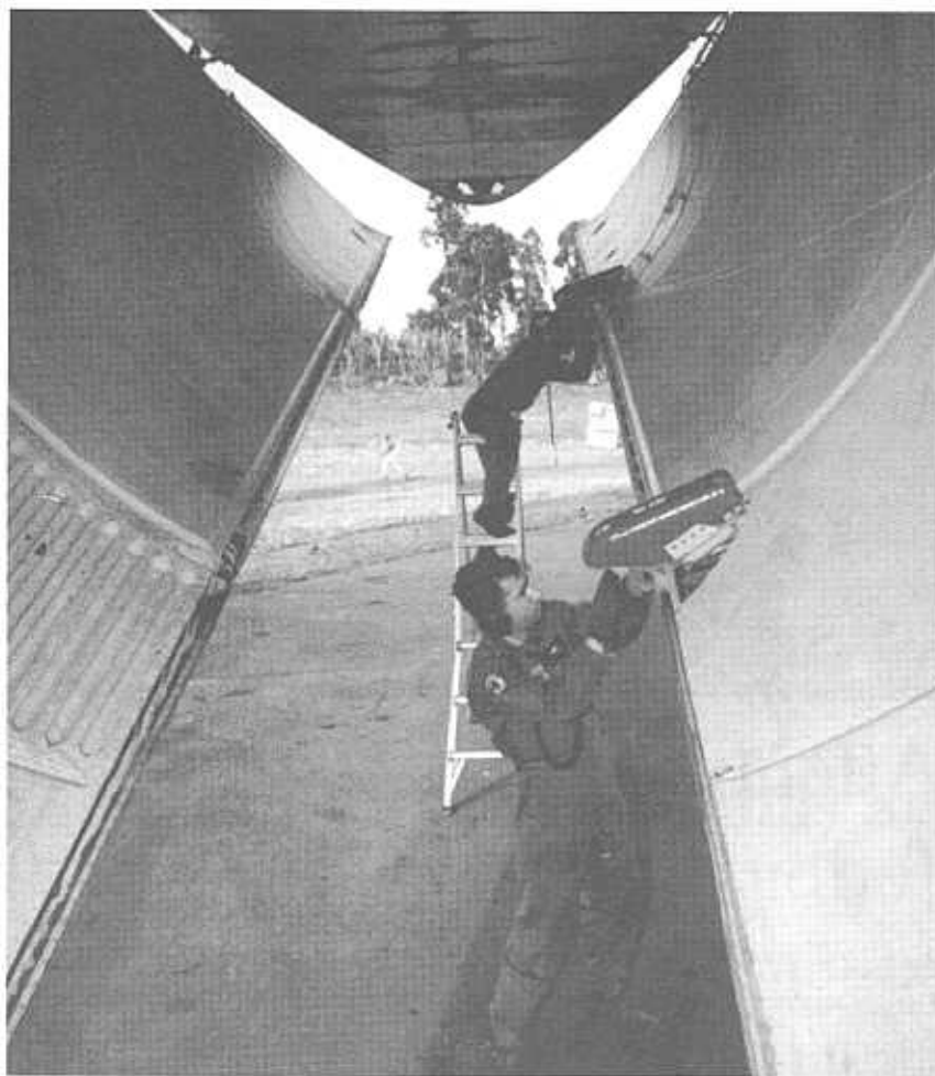
U.S. Army photo by Staff Sgt. Rolando Gomez. Staff Sgt. Bernie von Dauber III, foreground, and Staff Sgt. Arnold Smiley Jr. repair the cargo door on their C-141 Starlifter while on the ground at Goma, Zaire, after unloading forklift equipment. The two maintenance technicians, from McGuire AFB, N.J., are part of the U.N. mission to protect Rwandan refugees.
