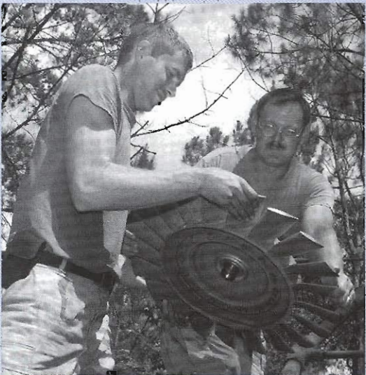
Pvt. Howard Fint (left) and Sgt. First Class Tony Robertson Fint lift a fan into place for an M88.
