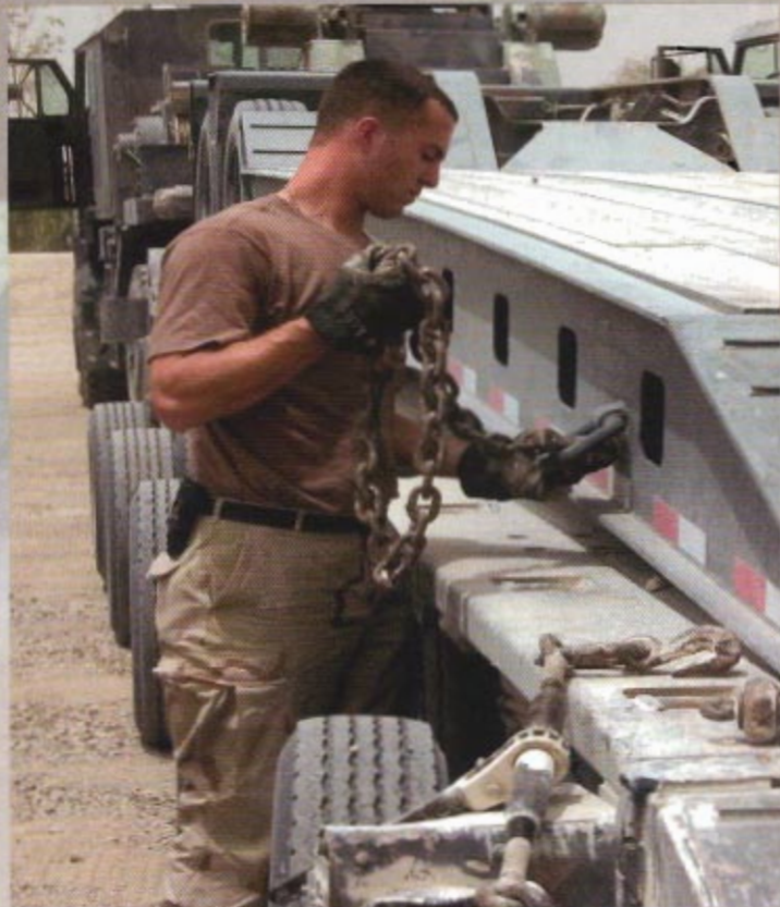
Spc James Frisby takes the time to tie down his load on the trailer of his HET.
