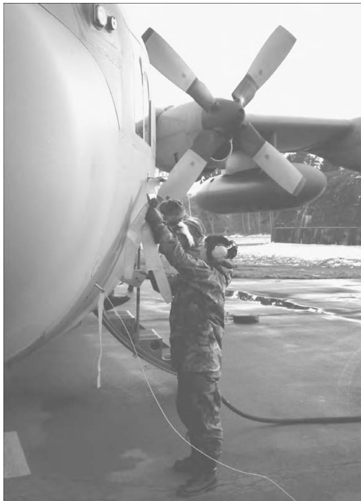
ABOVE: The Ohio Air Guard's Staff Sgt. Ron Anderson connects a generator cable to a C-130 at Ramstein Air Base, Germany.
