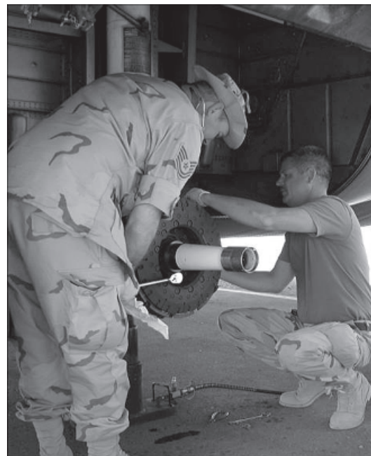
ABOVE: Tech. Sgt. Ron Thomas, right, of the 123rd Maintenance Squadron and another NCO work on the brakes of a C-130 Hercules at the deployed location.
