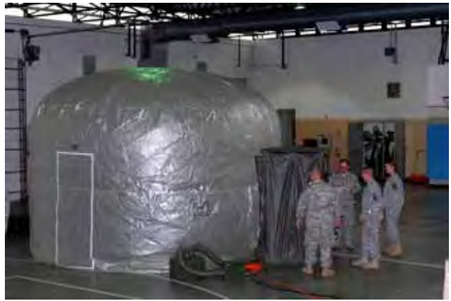
HHC 63 rd TAB Personnel conduct CBRNE training with a Collective Protection Equipment System.
