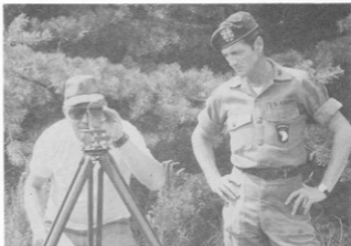
ON THE LEVEL —SSgt. Tom Neill, left, of Ashland's engineer unit, checks the elevation of an earth-moving project near Central City as Capt. Jimmy Napier, Army Advisor to the 201st Engineer Battalion, looks on. (Photo by SFC Keith Kappes)
