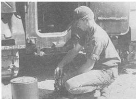
MAINTENANCE —SSgt. Orville Phillippi, of Somerset's mechanized infantry unit, changes the oil filter on an armored personnel carrier at Fort Hood. Maintenance was a major effort as the vehicles were tasked over difficult, very dusty terrain. (Photo by SP5 Tom Murphy)
