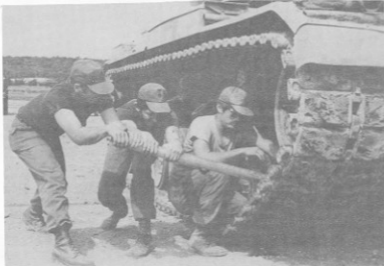
TRACK REPAIR —Three Madisonville Guardsmen work to replace a tank track link during annual training at Fort Hood, Tex. From left are SFC James Baxter, SSgt. Tony Space, and SP4 Joseph Hudson. See pages 2 and 3 for more AT photos. (Photo by SP5 Tom Murphy)
