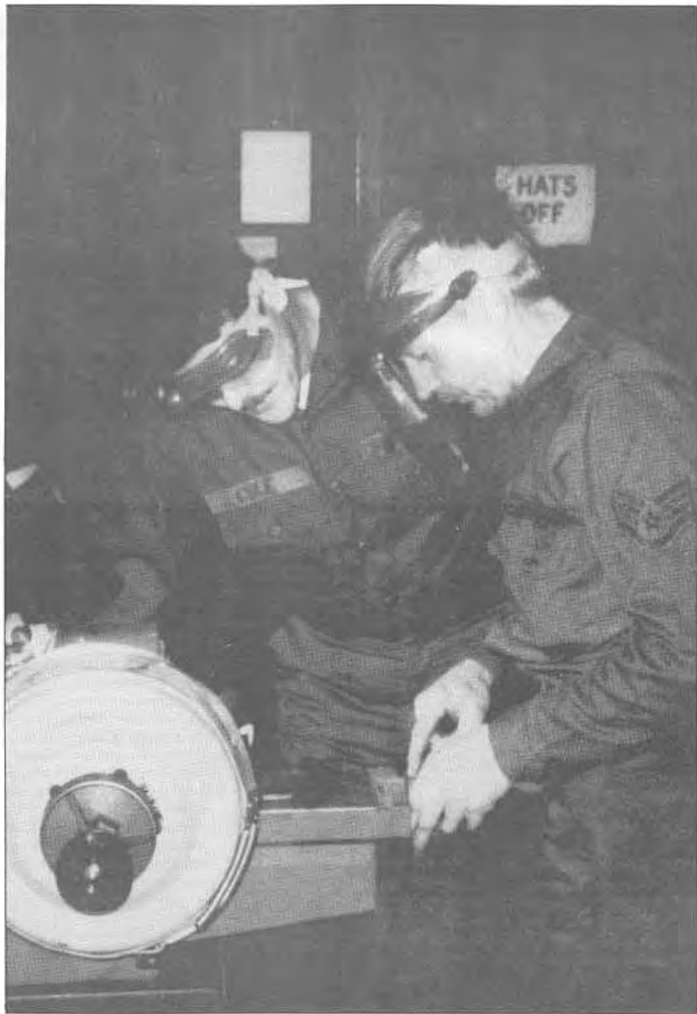
SSgt. Gary Cole, left, and SSgt. Benny Smiley, base motor pool, rotate brake drums.
