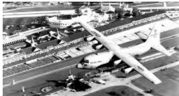
Using its aft loading ramp and door the C-130 can accommodate a wide variety of oversized cargo, including everything from utility helicopters and six wheeled armored vehicles to standard palletized cargo and military personnel. In an aerial delivery role, it can air drop loads up to 42,000 pounds or use its high-floatation landing gear to land and deliver cargo on rough, dirt strips.
