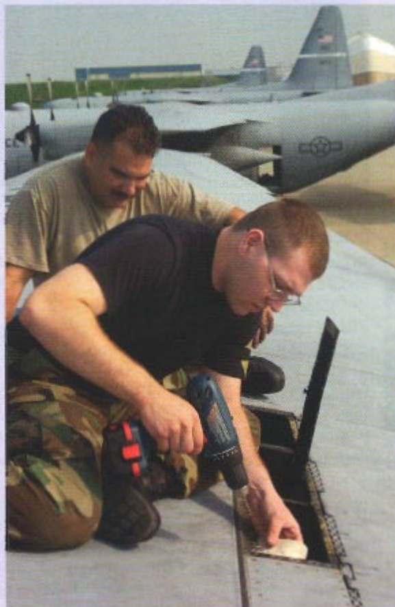
Senior Airman Lee Stanley and Tech. Sgt. Carl Shaffer, both members of the 123rd Maintenance Group, replace a nutplate on a C-130 Hercules here. (Photo by Senior Airman Phillip Speck/KyANG)
