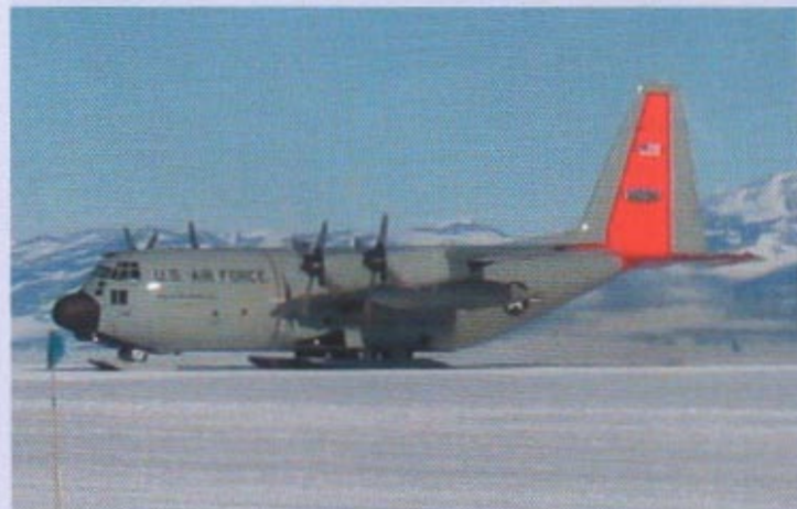
Airlift into and out of McMurdo Station is provided by the New York Air Guard's LC-130 transport aircraft, which feature modified landing gear. Special skis have been fitted to the planes' wheels to allow for landings on packed ice. (Photo courtesy Senior Master Sgt. Barry Wright.)
