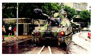
This M109A5 155mm Self Propelled Howitzer is used for indirect fire support. It fires an approximately 6.2 inch diameter shell up to 14.5 miles.
