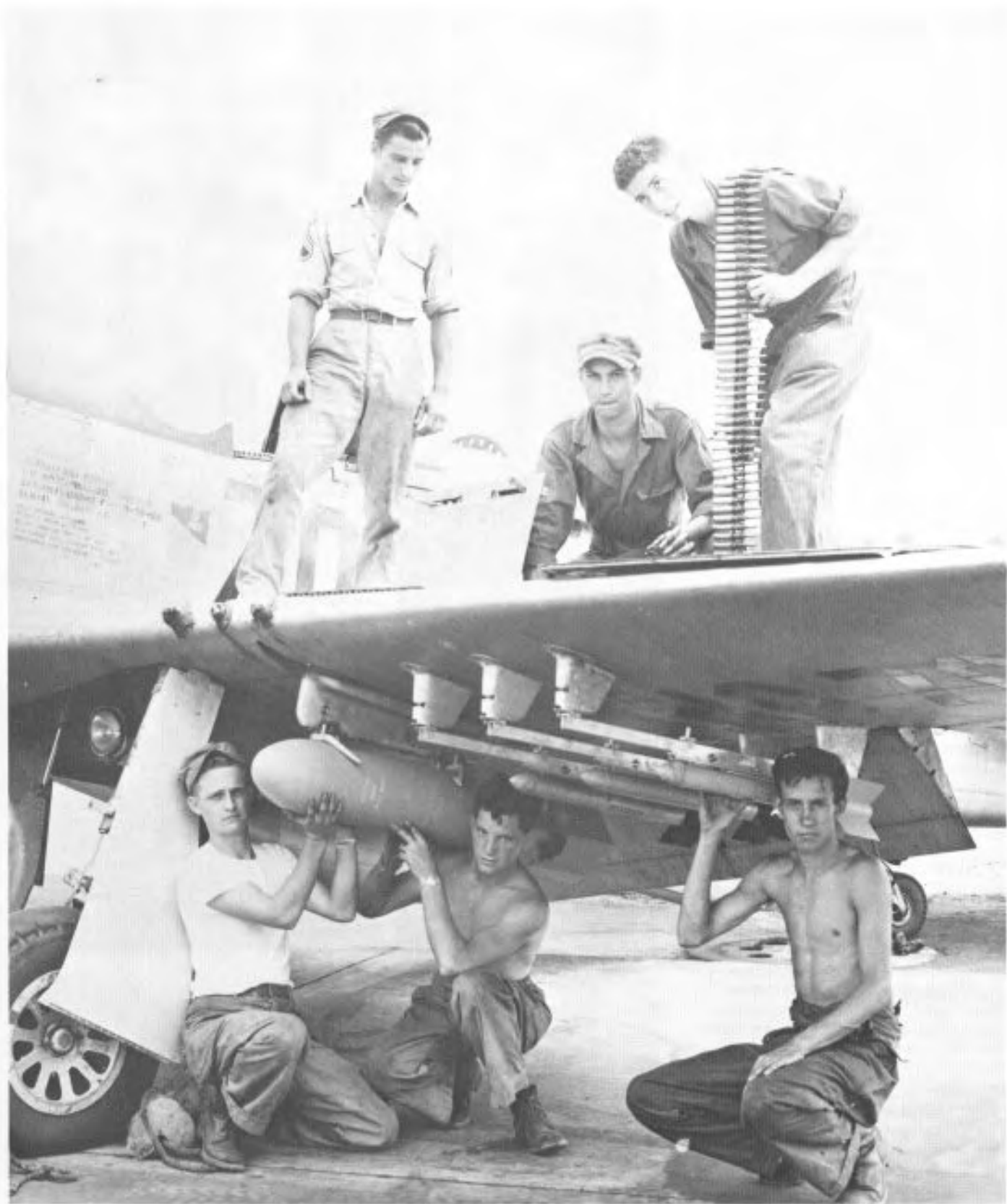
LOADING AMMO: The 25 F-51 Mustangs of the 123d Fighter Group were almost new when they were received at Standiford Field. They were D-model Mustangs, equipped with six rockets, a pair of 500-pound bombs, and six .50-cal. machineguns. Members of the maintenance crew were obviously impressed with the armament of the Mustang. Unfortunately the identification of many of the early Air Guardsmen has grown dimmer over the years, but Carl Bundschu (left) and John Mulhall (right) are on top of the wing and Arvel Lindsey (right) is holding a rocket.
