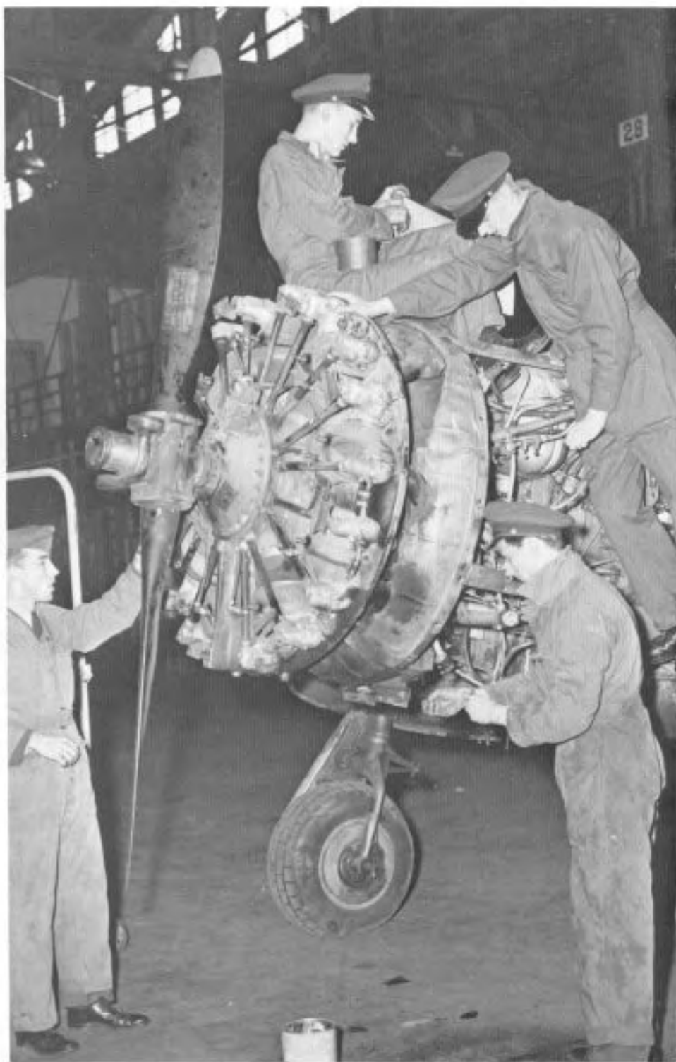
TEXAN MAINTENANCE: The first aircraft owned by the Kentucky Air National Guard were T-6 Texans. Here, inside the old Hangar Building, maintenance personnel work on one of the radial air-cooled engines of the most widely used type of trainer ever flown. The two men standing on the floor are Tom Rogers (left) and Leroy Martin (right).
